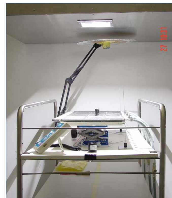
Figure 3. The 6500 W Xenon Arc Solar Simulator used in the in vitro phototoxicity assays. Note the custom cooling bed that is used to minimize cell heating and maintain a constant temperature during UVA exposure.
