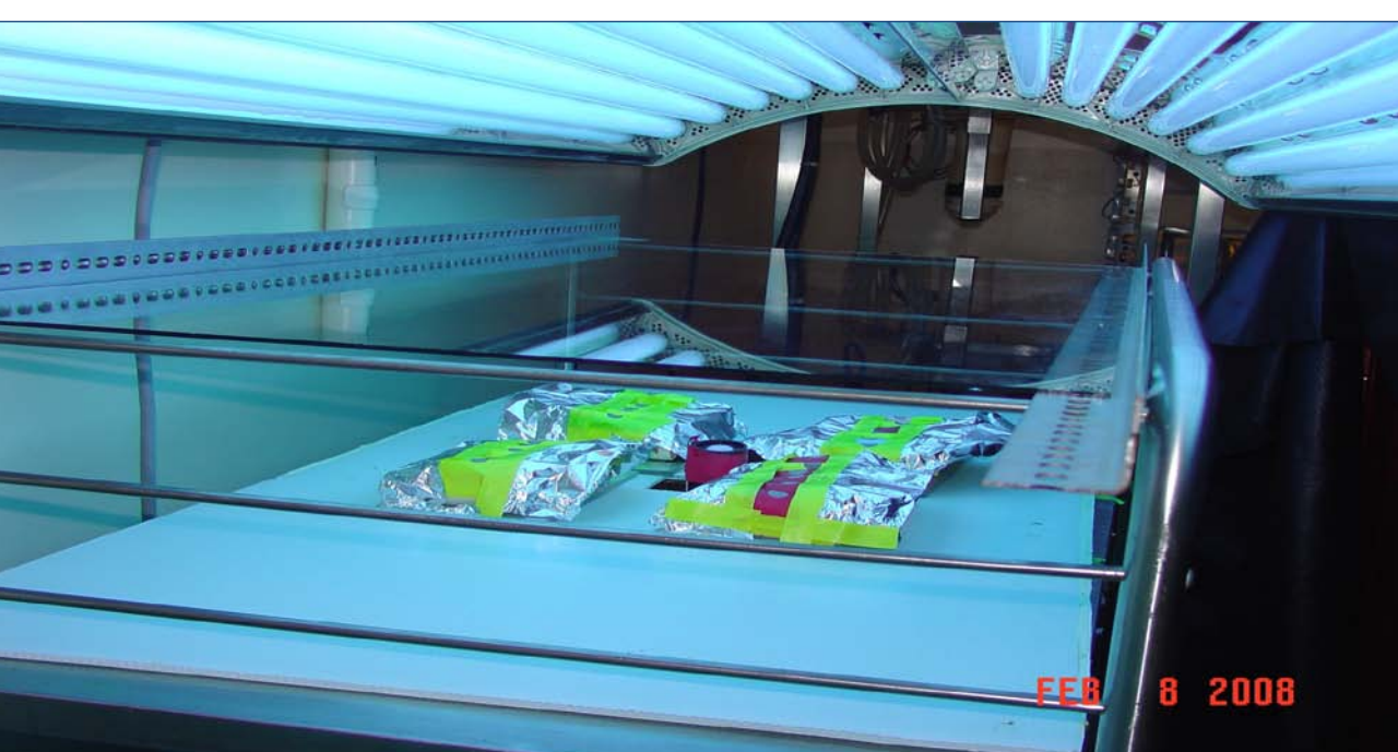
Figure 1. Fluorescent fixture (KBD, Inc) used in the maximized in vivo phototoxicity test to allow for delivery of a relative high dose of UVA (315 – 400 nm).
